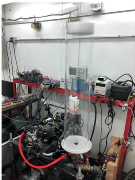
Figure 2 Engine setup and exhaust gas collection system
